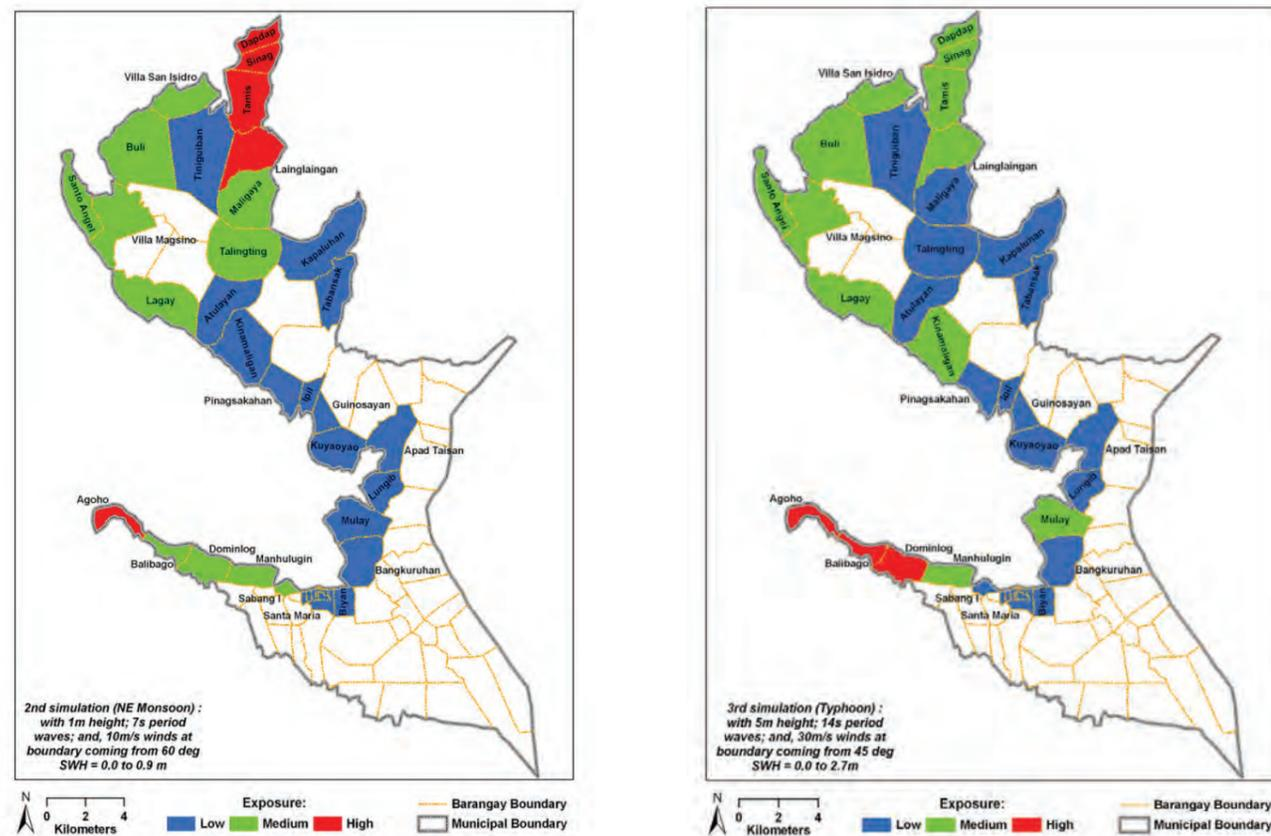
Figure 16: Wave exposure during NE winds (left) and typhoons (right). Scores of 1-3-5 are assigned respectively to low (L), medium (M), and high (H) exposure to waves
