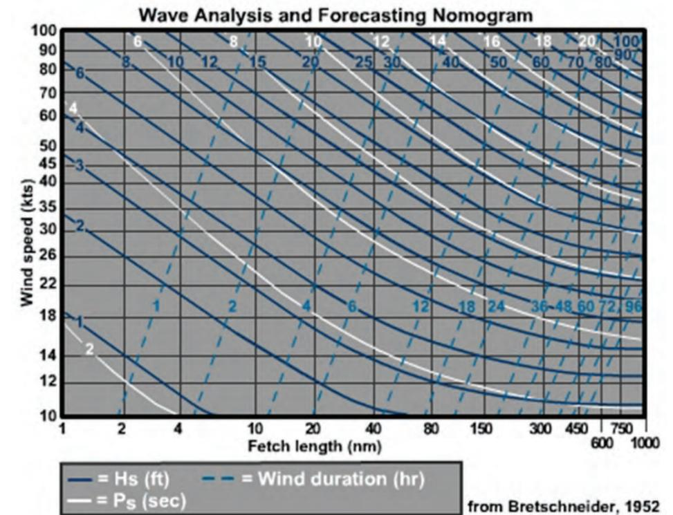
Figure 3: Wave analysis and forecasting nomogram (from Bretschneider, 1952)
