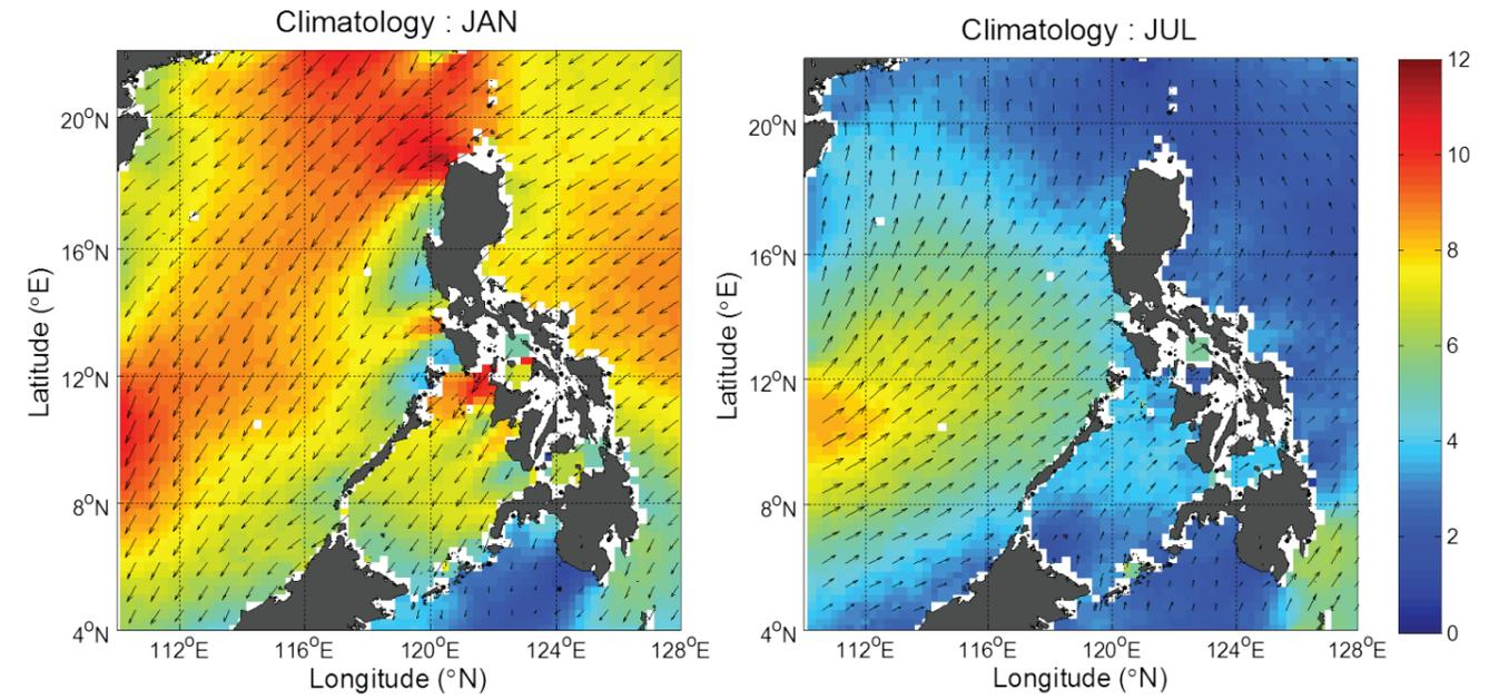
Figure 5: Wind climatology or pattern for the Philippines based on the 10-yr QUIKSCAT dataset. Colors denote speed (in m/s) while arrow length and angle denote magnitude and direction of wind vectors
